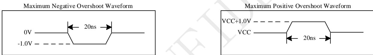
Figure 5-2 Input Test Waveforms and Measurement Level
